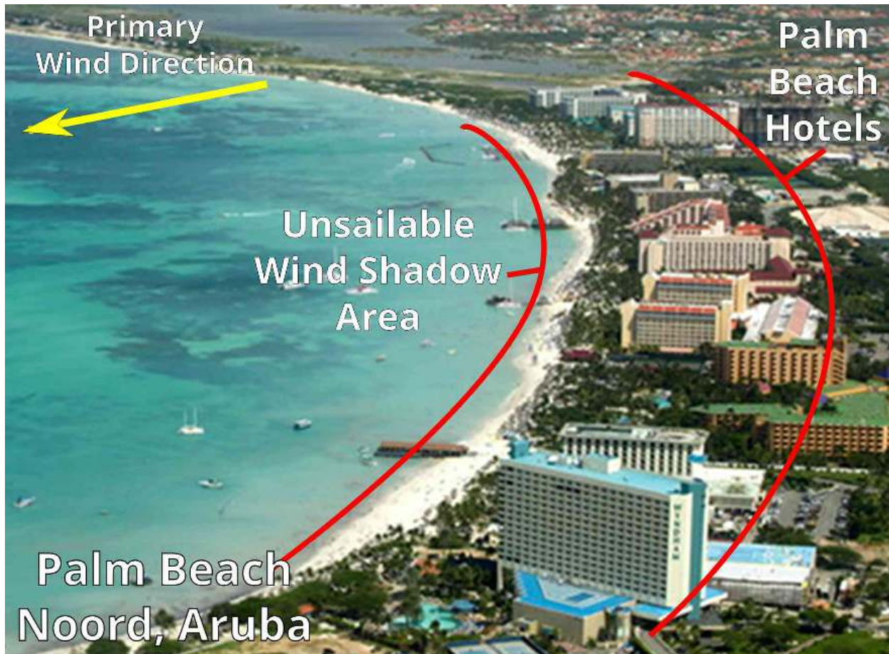
Figure 6: One of the world’s formerly-leading windsurfing destinations is located in Aruba. In the early 2000’s, a series of commercial developments changed the wind patterns dramatically. The sailing area is now a fraction of what it was. This well-known case is very comparable to the Baylands but was not considered in the EIR, though the EIR consultant was informed of it.
